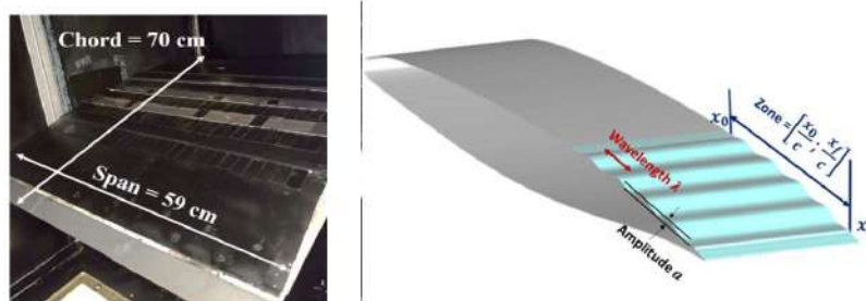
Figure 1: “Live-skin” embedded on the subsonic “Intermediate Scale - IS” A320 morphing prototype (left), in the S4 wind tunnel of IMFT. Right: Schematic visualisation of the wavy surface modelling the present actuation.
