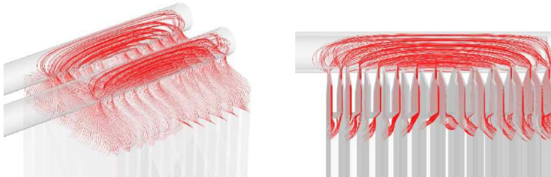
Figure 1: Visual representation of ionic current streamlines (stray currents) in channels and manifolds
