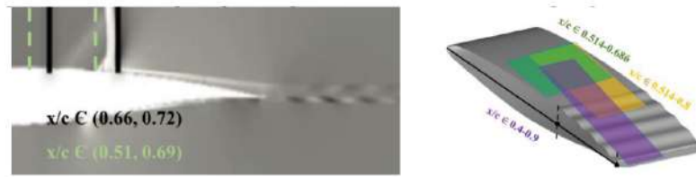
Figure 2: Left – Visualization of the maximum upstream and downstream positions of the shock wave in the static (non-actuated) case, located between x/c = 0.66 and x/c = 0.72 . The green area (dashed vertical lines) corresponds to an optimal actuation zone indicated on the right. Right – Schematic representation of the various travelling wave (TW) actuation zones tested in the continuation study, covering regions upstream of the shock as well as zones that extend across and beyond the shock excursion envelope.
