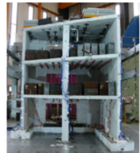
RC specimen of SMART2013 anchored on the AZALEE shaking-table
